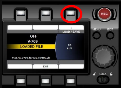
5. Select 3D LUT again and Press LOAD and then select from list on SD Card. Press Dial to load selection.
